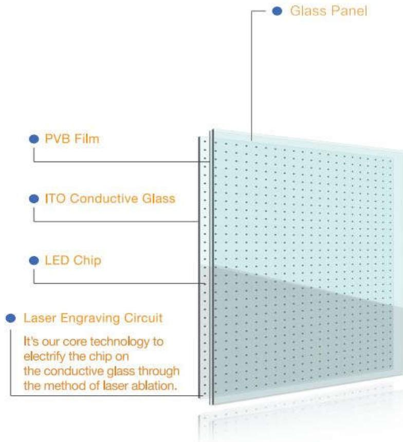
Wooscreen glass display is composed of ITO conductive glass, glass panel and LED chip. We use laser to sculpture the circuit to realize image, animation, text and video playing.
